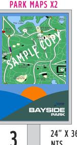
24" X 36" NTS VERTICAL MOUNT WITH FRAME 60" FROM GRADE TO **CENTER OF SIGN**
